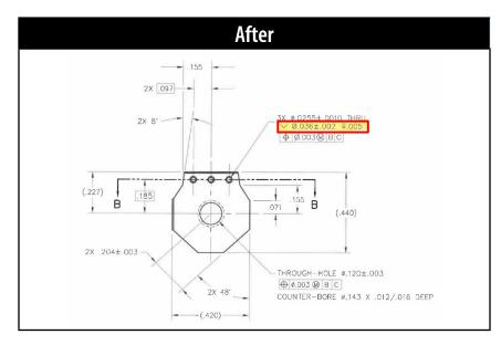
There is no change to the form, fit, function or quality of the affected part numbers. The reliability of the affected part numbers will improve due to better flow of resistive ink after the ink depth is reduced. Traceability will be maintained through lot code and date code.
