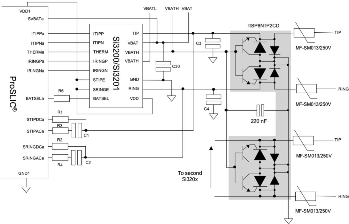
Figure 10: TISP6NTP2CD to protect dual port applications to GR-1089-CORE intra-building.
