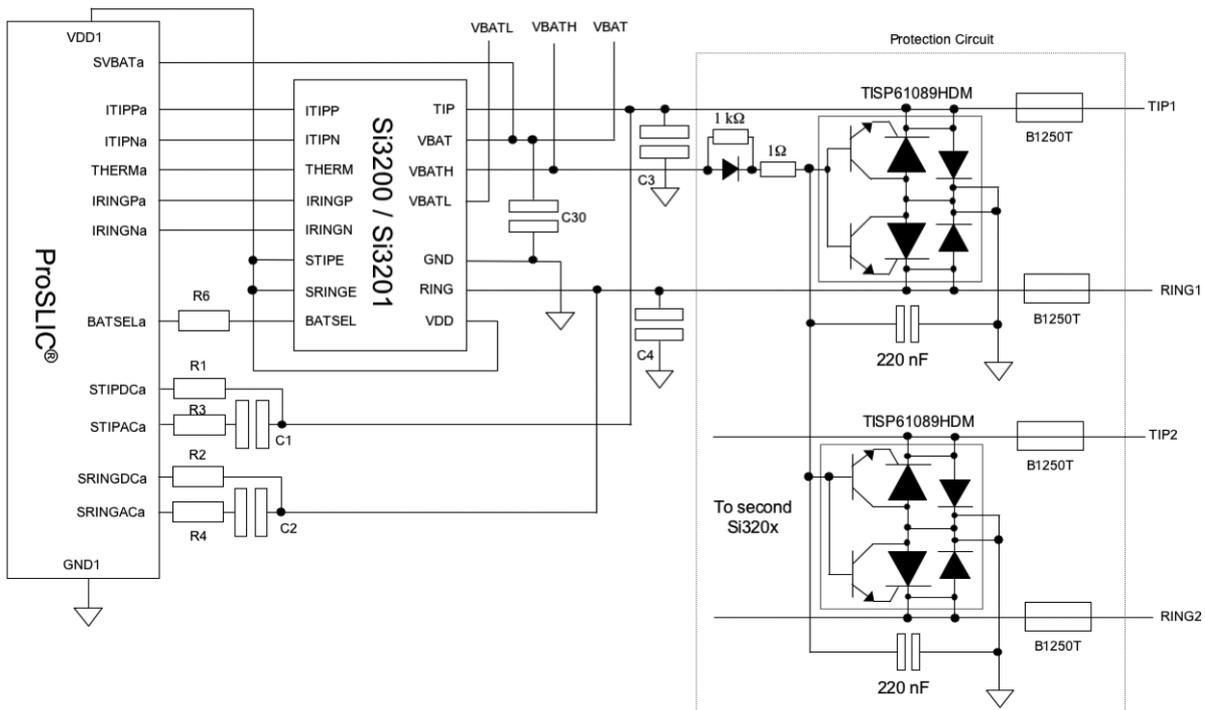
Figure 9: Si320x protection for Telcordia GR-1089-CORE applications
