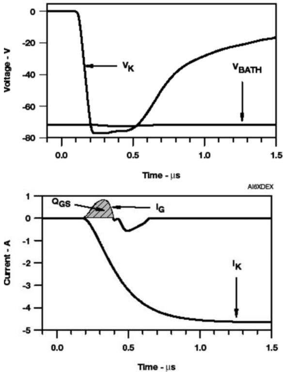
Figure 8: Gated thyristor switch characteristics
