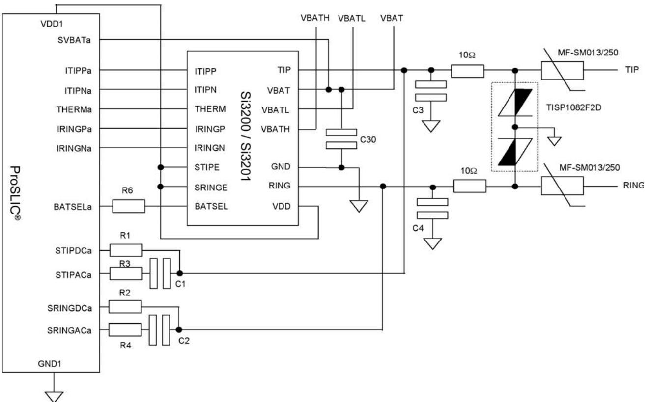
Figure 5: Si3200 and Si3201 integrated line driver for intra-building applications
