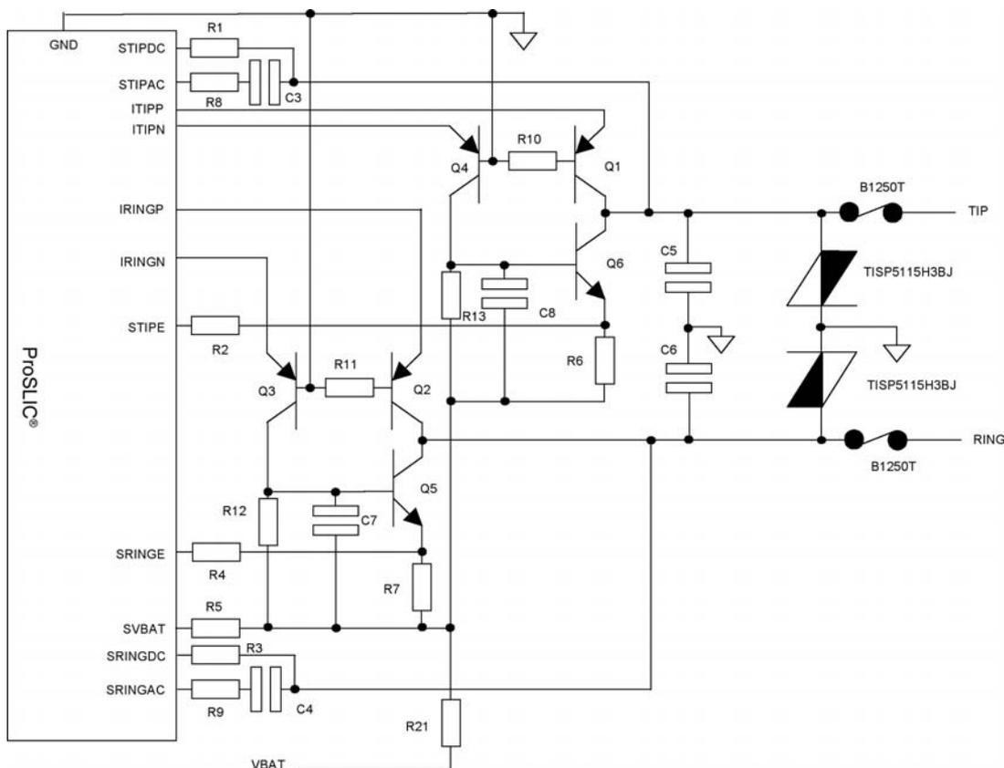
Figure 4: Si3210 ProSLIC® with discrete line driver with protection
