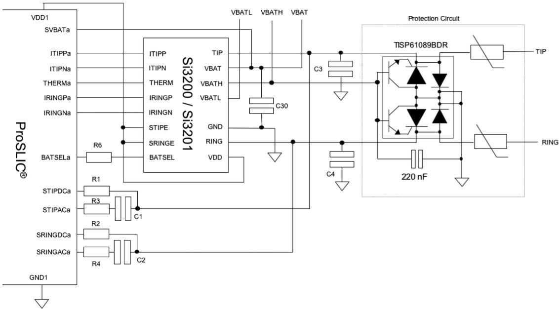
Figure 11: TIA-968-A and UL 60950 protection for Si320x line drivers
