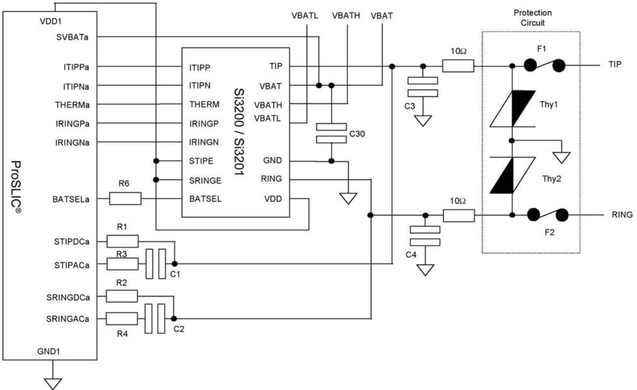
Figure 2: Si3220 ProSLIC® with Integrated Line Driver and Protection
