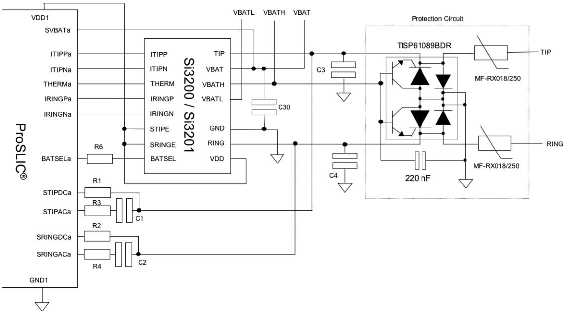
Figure 12: Basic ITU-T protection for Si320x line drivers
