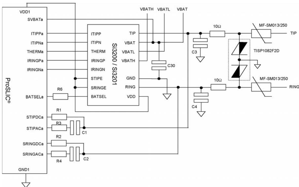
Figure 7: Si3200 and Si3201 for ITU-T basic and enhanced applications
