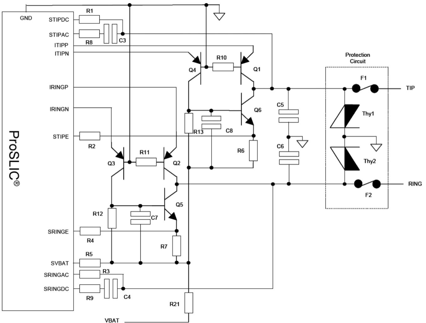
Figure 1: Si3210 ProSLIC® discrete line driver with protection
