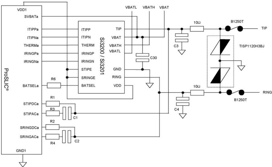
Figure 3: Si3220 ProSLIC® with integrated line driver for GR-1089-CORE applications
