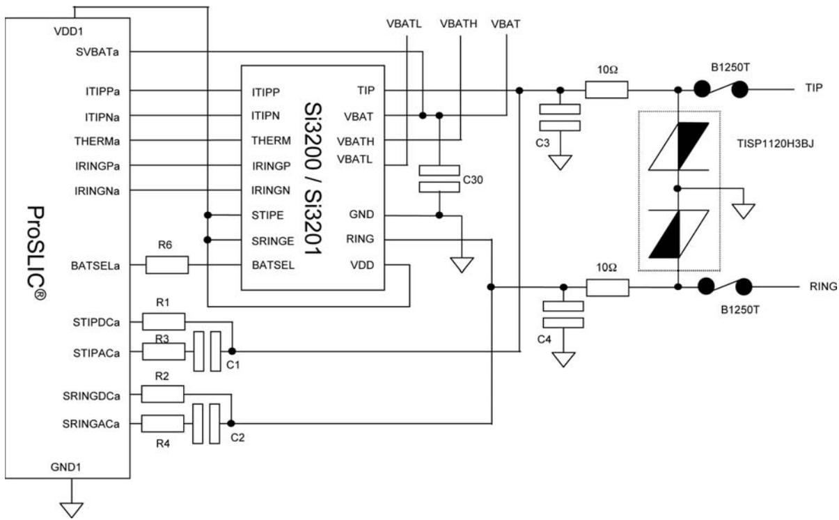
Figure 6: Si3200 and Si3201 protection solution for TIA-968-A and UL 60950 applications
