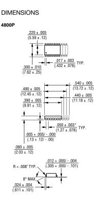
Lead coplanarity .004 inch max. at mounting surface.
