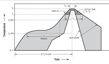
Ramp-up rate = 3 °C/sec. max. Ramp-down rate = 6 °C/sec. max.  $T_L = 217 °C$   $t_L = 60-150 sec.$   $T_p = 245 °C \pm 5 °C$ Time within 5 °C of actual Peak Temp  $(t_p) = 20$ ~40 sec.  $T_S min = 150 °C$  Ts max = 200 °C  $T_S min to T_S max = 60-180 sec.$ , 25 °C to Peak Temperature = 6 min. max.
