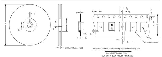
В С D G N Α Min. Max. Min. Max. Min. Max. Min. Max. Ref. Ref. 330 1.5 2.5 12.8 13.5 20.2 326 16.5 102 (13.002)(.059)(.098)(.650)(12.835)(.504)(.531)(.795)(4.016)
