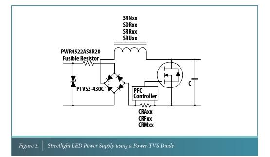
Figure 2 is a representation of how a typical streetlight LED power supply may be configured using a Power TVS diode (PTVS) instead of a more common varistor to protect against transients in this electrically-exposed environment. Completing the power supply design, Bourns has a broad selection of inductors available in high current, flat wire, semi-shielded and fully shielded options to maximize performance.
