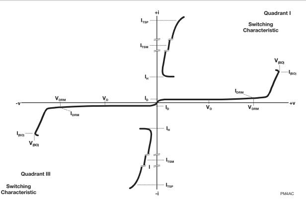
Figure 1. Voltage-Current Characteristic for any Terminal Pair
