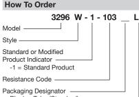
Blank = Tube (Standard) R = Tape and Reel (X and W Pin Styles
