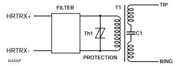
Figure 13. Home Phone Networking Isolation/filter/protection Circuit
