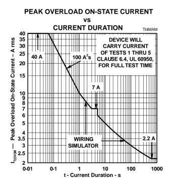
Figure 4. Peak Overload On-state Current against Duration
