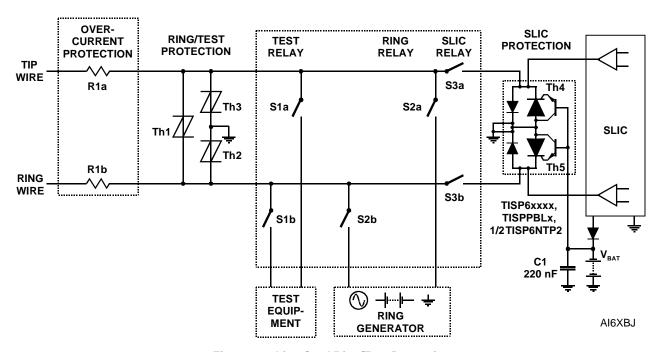
Figure 17. Line Card Ring/Test Protection
