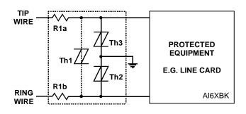
Figure 14. Modem Inter-wire Protection
