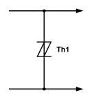
Figure 12. Two Point Protection
