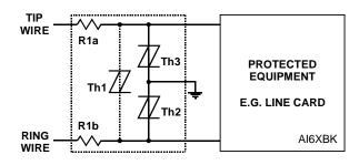
Figure 14. Modem Inter-wire Protection
