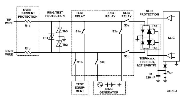
Figure 17. Line Card Ring/Test Protection
