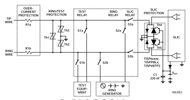
Figure 18. Line Card Ring/Test Protection
