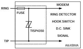
Figure 15. Modem Inter-Wire Protection
