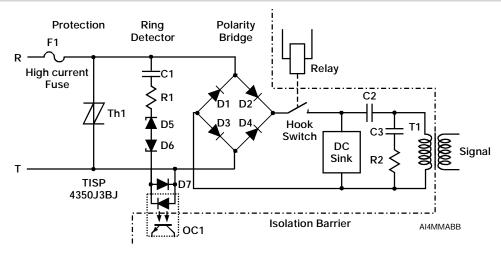
Figure 8. Typical Application Circuit
