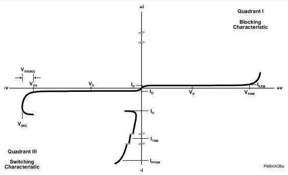
Figure 1. TISP8210MD KA Terminal Characteristic
