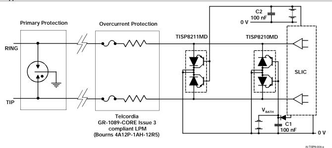
Figure 3. Typical Application Circuit
