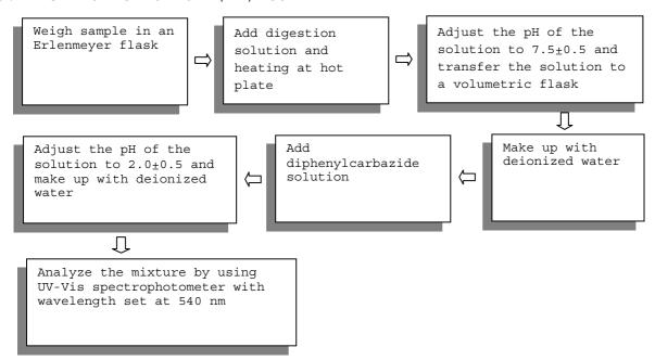
4. TEST FOR CHROMIUM (VI) CONTENT (BOILING WATER EXTRACTION ON METAL)
