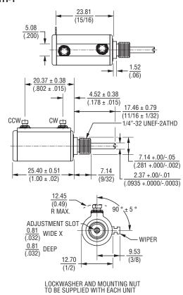
$\begin{array}{ll} \text{TOLERANCES: EXCEPT WHERE NOTED} \\ \text{DECIMALS: .XX} & \underline{.25} \\ \underline{(.010)} & .XXX & \underline{.13} \\ \hline \text{FRACTIONS: } 1/64 \\ \text{DIMENSIONS: } \frac{\text{MM}}{\text{(IN)}} \\ \end{array}$
