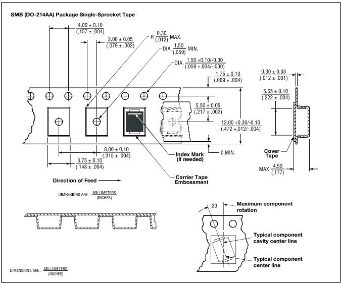
NOTES: A. The clearance between the component and the cavity must be within 0.05 mm (.002 in) MIN. to 0.65 mm (.026 in) MAX. so that the component cannot rotate more than 20 ° within the determined cavity.
