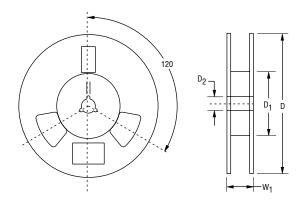
Devices are packed in accordance with EIA standard RS-481-A and specifications shown here.
