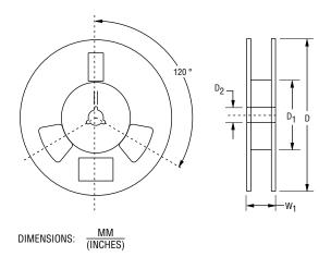
Devices are packed in accordance with EIA standard RS-481-A.
