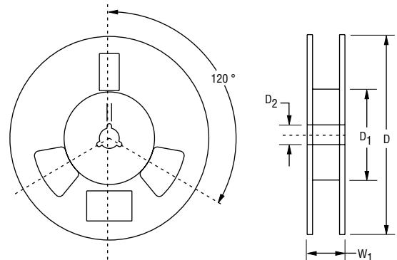
Devices are packed in accordance with EIA standard RS-481-A.
