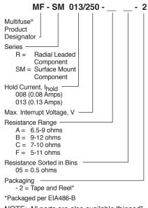
NOTE: All parts are also available "binned". All parts within a package will be within 0.5 ohms of each other within the initial resistance range.
