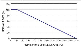
These resistors must be attached to a suitable heat sink. The maximum internal resistor temperature is +175 °C.
