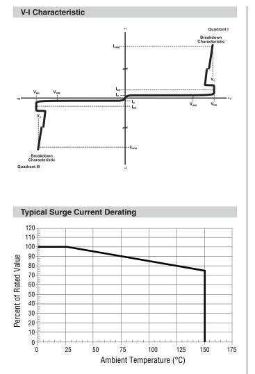
This graph shows the typical device surge current derating versus ambient temperature when subjected to the  $8/20 \,\mu$ s current waveform per the IEC 61000-4-5 specification. This device is not intended for continuous operation at temperatures above 125 °C.
