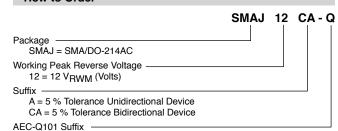
Q = AEC-Q101 Compliant, 13-inch Reel QH = AEC-Q101 Compliant, 7-inch Reel (available only for 12 V to 58 V models)
