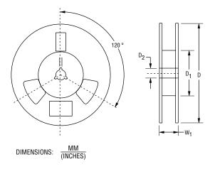
Devices are packed in accordance with EIA 481 standard specifications shown here.
