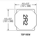
† Dimension does not include termination. For maximum overall dimensions with termination, add 0.1 mm (.004 in.).
