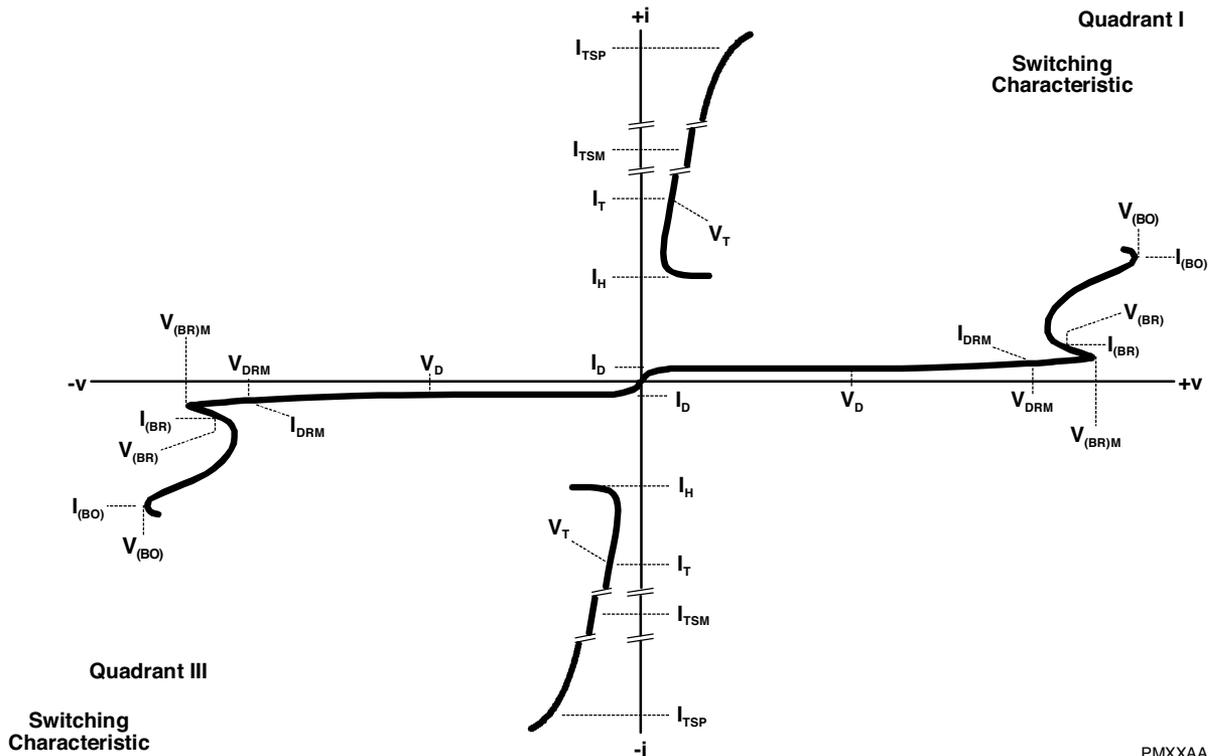
Figure 1. Voltage-Current Characteristics for any Terminal Pair
