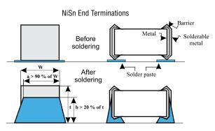
Fig. 5 Soldering Criteria for Wave and IR Reflow Pb-free Soldering
