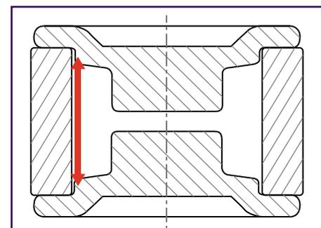
Figure 6. | Cross Section of a Typical GDT
