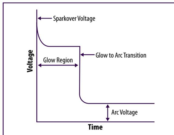
Figure 3. | General Operation of a GDT
