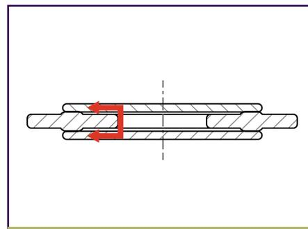
Figure 7. Cross Section of a FLAT® Technology GDT
