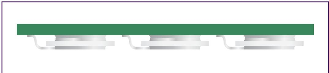
Figure 10. | Example of Horizontally Mounted Bourns® FLAT® GDTs
