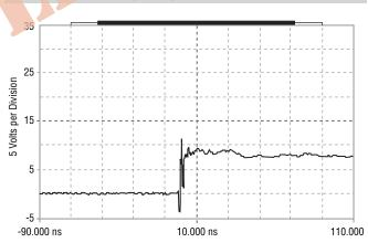
ESD Test Pulse - 25 kilovolt, 1/30 ns (waveshape)
