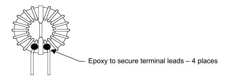
This product quality improvement process will be implemented on selected part numbers of the 7100 series chokes that are wound with 0.5 mm or finer diameter wires. Without epoxy, smaller diameter wire leads tend to reposition during transportation and next-level assembly handling.
