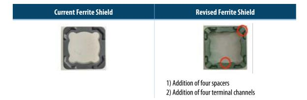
In addition, the core-to-mounting base assembly will change from a manual to a semi-automated process.
