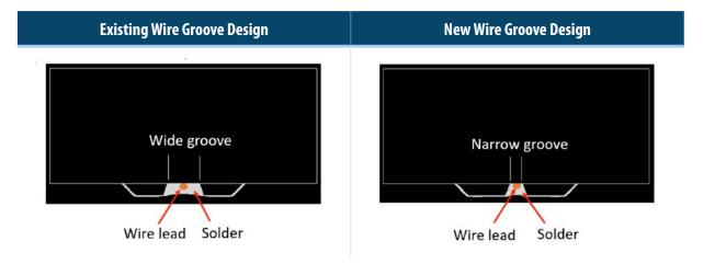
The form of the inductor will change because of the narrower wire groove. The fit and function of the inductor will remain the same. The quality and reliability of the component should be improved.
