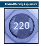
The form of the inductor will change due to the change in the marking method. The fit and function will remain the same. The quality and reliability should be improved as the result of the manufacturing process change.
