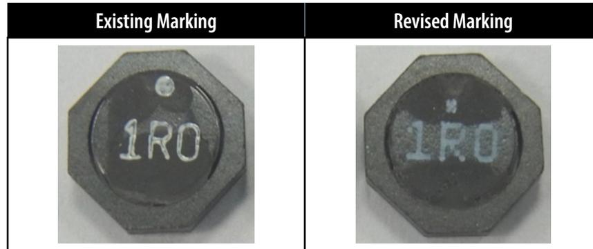
The new marking process will increase marking durability and reduce the chemical impact on the environment.
