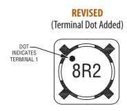
On the data sheet, the terminal number assignment (shown below) will be rearranged to align with the Terminal 1 marker. These numbers are not marked on the actual part.
