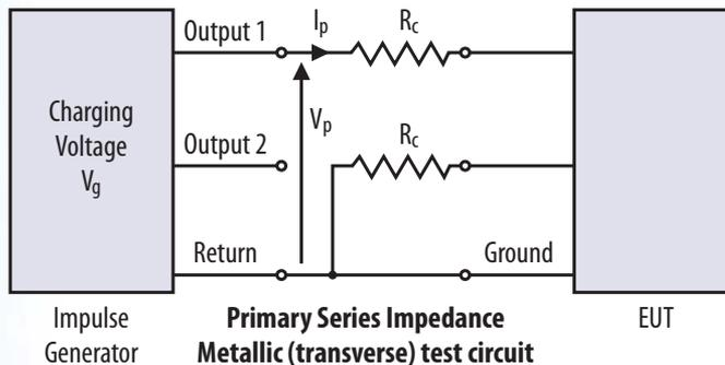
**Figure 3. Test Circuit for fitted primary protector configuration**
