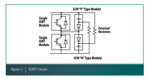
For the external resistors, thick film SMD resistors such as Bourns<sup>®</sup> Models CRM2512, CRM 2010, CRM1206, and CRM0805 have good surge capability and are available with power ratings up to 2 W. Thick film non-inductive resistors are available up to 35 W including Bourns<sup>®</sup> Models PWR163 and PWR263 in DPAK packages and Bourns<sup>®</sup> Models PWR220T and PWR221T in TO-220 packages.
