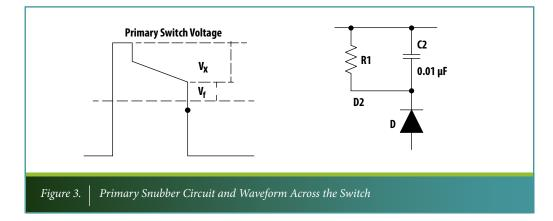
The flyback voltage is generated by the secondary winding coupling its voltage to the primary winding during the off time of the switch. Due to the turns ratio this voltage can be quite high. The sum of the clamped voltage and the flyback voltage must be kept below the maximum rated  $V_{ds}$  of the switch.
