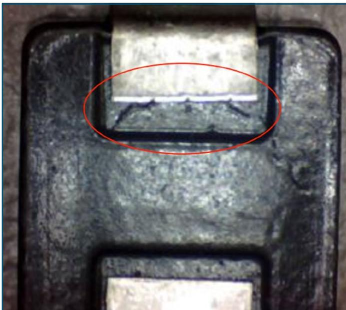
Figure 3 | *Acceptable Crack*
