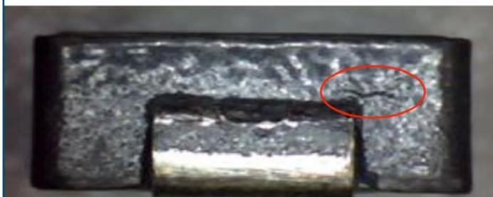
Figure 7 | Acceptable Crack
