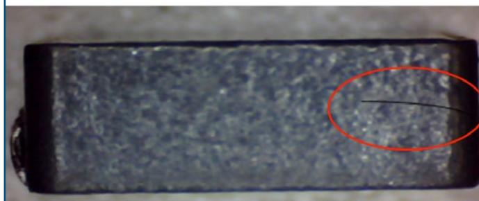
Lateral crack: Crack covers less than 50 % of the length of the side.
