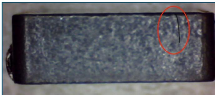
Vertical crack: Crack does not extend from one side to another.
