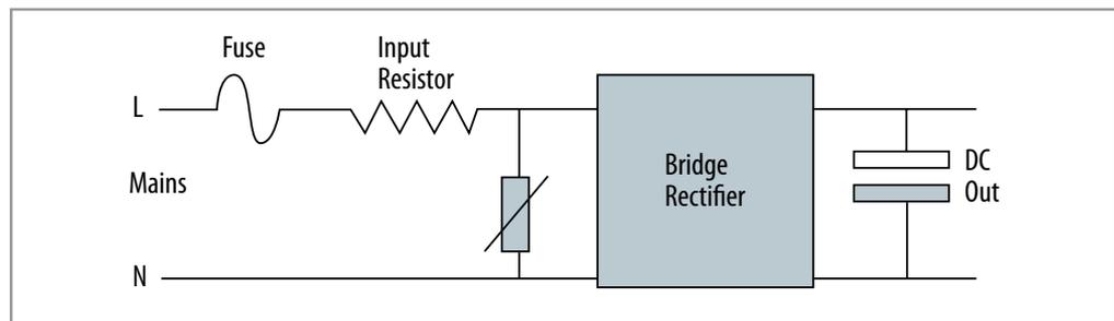
Figure 2 | Typical Inrush Current Limiting Circuit
