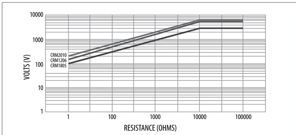
Figure 1 | Bourns® CRM Pulse Characteristics
