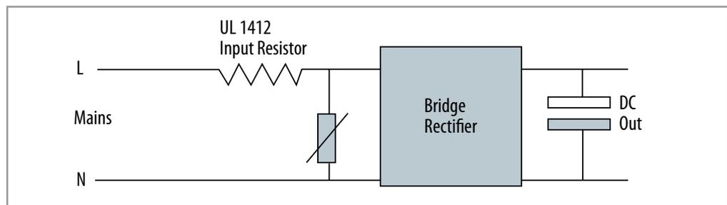
Figure 3 | Integrated Inrush Current Circuit
