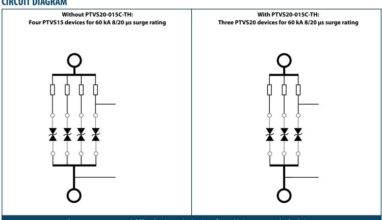
Fewer components on each PCB and easier production, i.e., reflow soldering - creates value for designers
