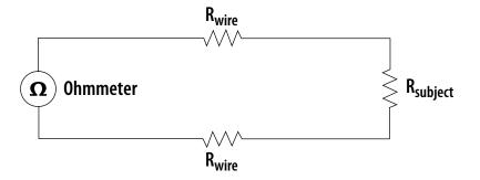
R measured =  $R_{wire} + R_{subject} + R_{wire}$
