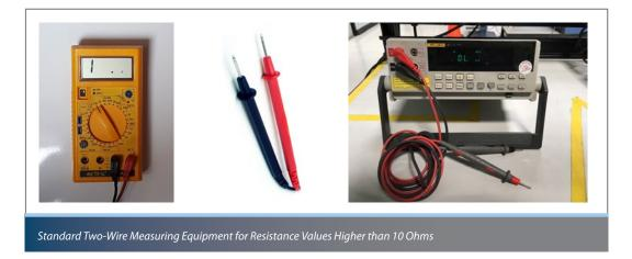
This method is also sensitive to contact probe failure or cable failure, and will introduce additional errors if those problems exist. The measurement of lower resistance values under 10 ohms using this method likely will be inaccurate, especially for metal strip current sense resistors with resistance ranges of 50 micro ohms to 100 milliohms. Therefore, with this method the lower the resistance value being measured, the more inaccurate the measurement results.
