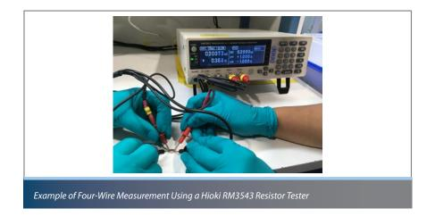
Since the voltmeter internal resistance trends to infinite, the measuring current is very small, typically 10 to 100 pA. Thus, the voltage drop on the current sense wire is very low compared to the voltage drop on the subject component forced by the main current. This is the reason that the resistance of the current sense wire has no significant influence on the measuring result.
