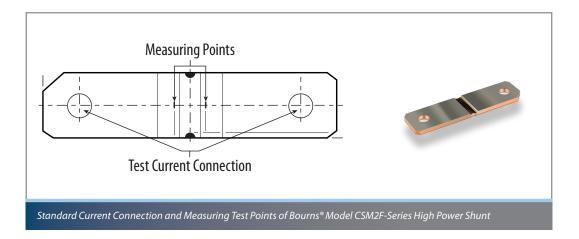
Bourns uses a Hioki RM3543 measuring instrument for metal strip current sensing resistors which is suitable down to µohm level.
