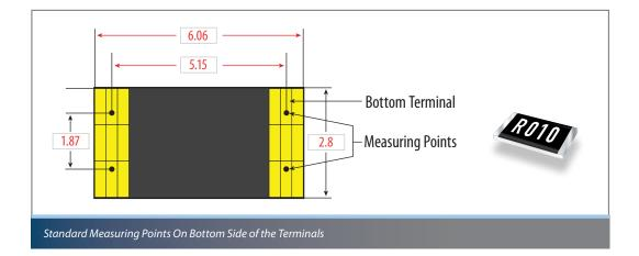
For the low resistance measurement Bourns uses a four-wire jig, which helps ensure that components are measured on the standard measuring points.
