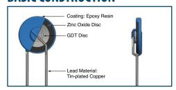
A GMOV™ component functions as the GDT isolates the MOV from the circuit until such time as the voltage exceeds the turn-on voltage of the GDT.
