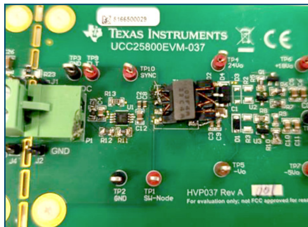
Figure 2. | Transformer mounted on driver board
