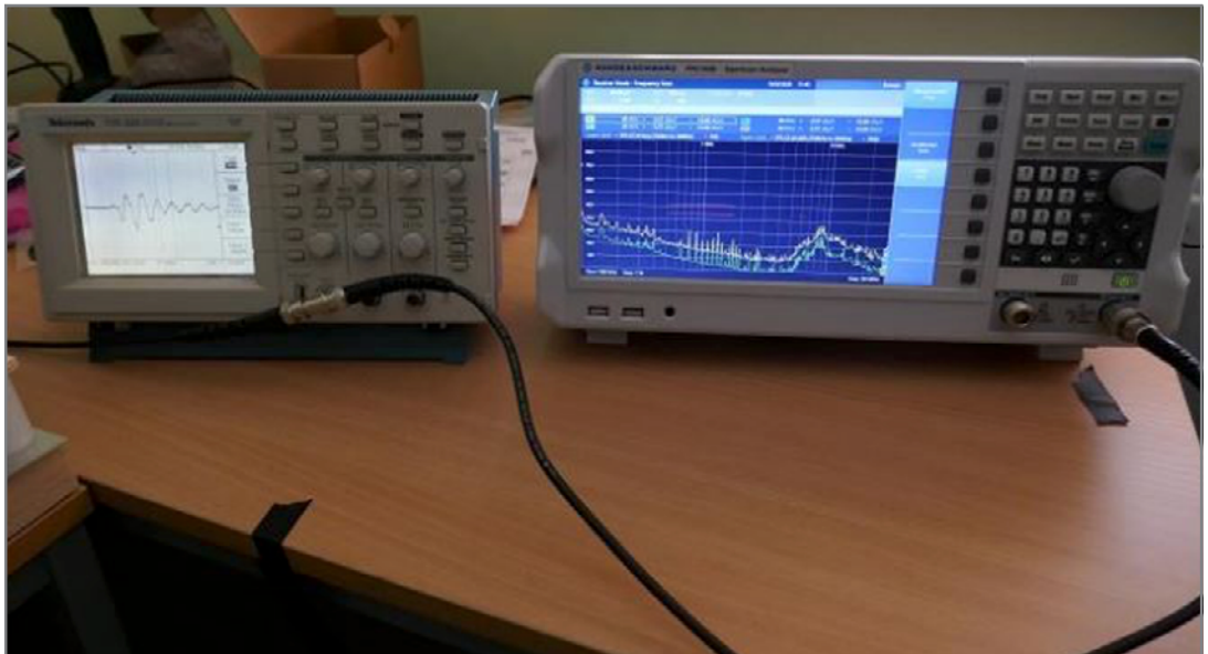
Figure 7 - Conducted emissions set-up showing scope and spectrum analyzer
