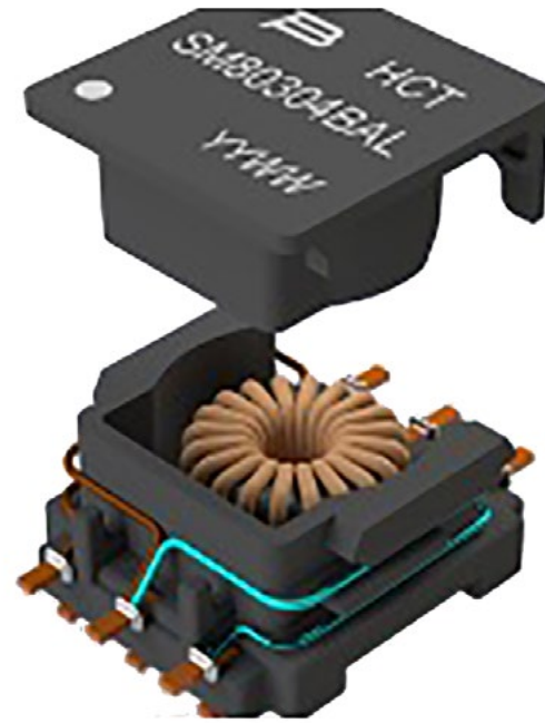
Figure 3: The construction of the Bourns Model HCTSM8 transformer with a toroidal core showing the lid and primary wire wrapped around the housing to extend the distance from the pins to the core
