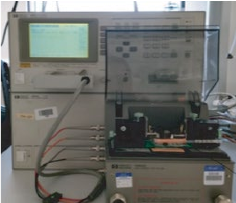
Figure 5: Photograph of the test fixture used to measure core loss
