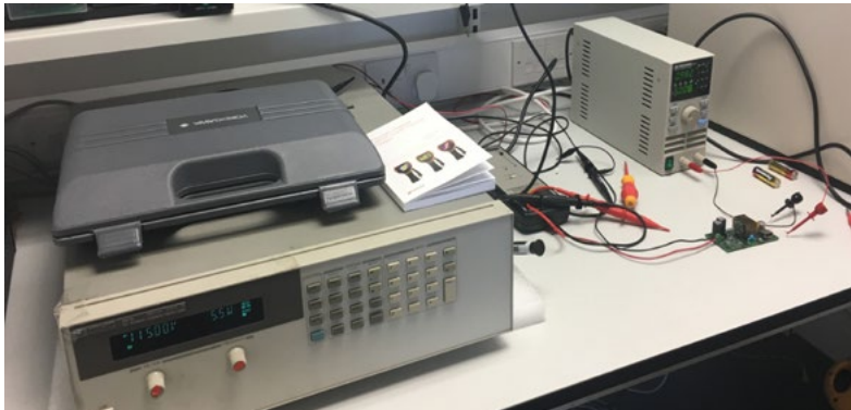
Figure 10: Test bench showing input and output power (91.05% efficiency)
