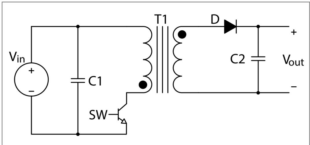
Figure 1 - Flyback converter schematic
