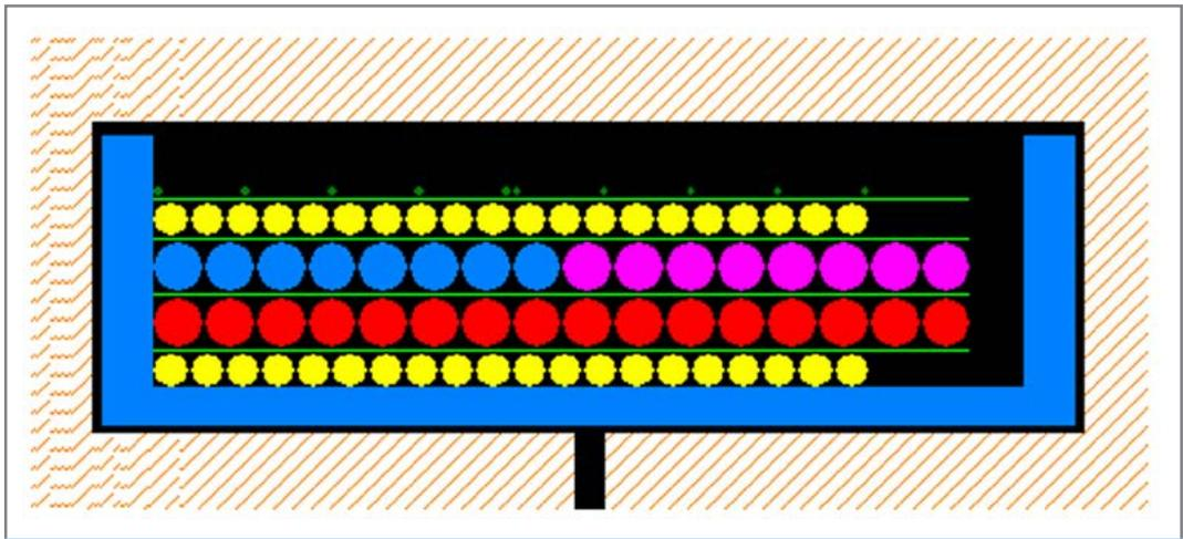
Figure 8 - Design 4 winding construction
