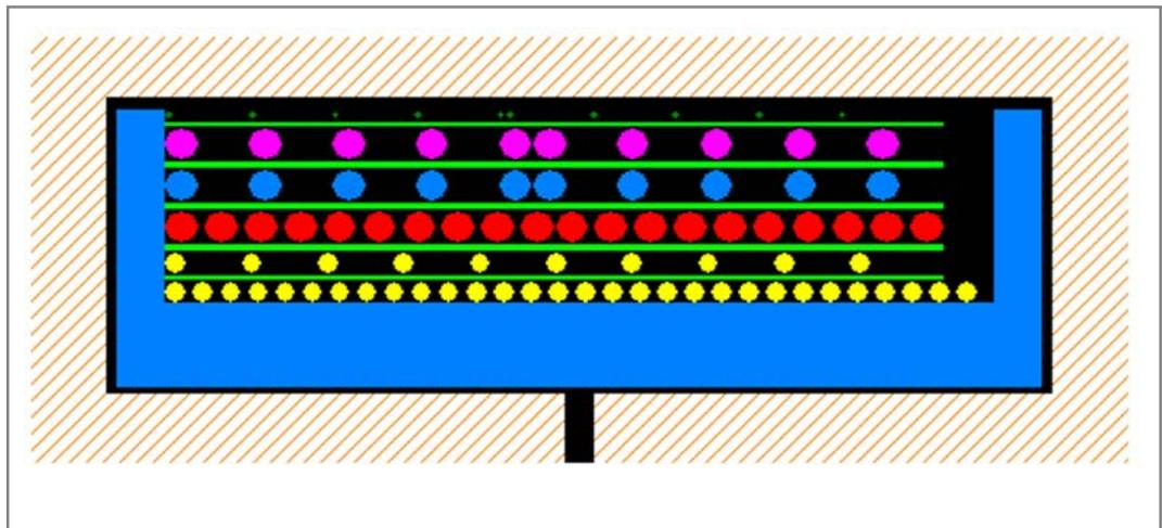
Figure 5 - Design 2 winding layout
