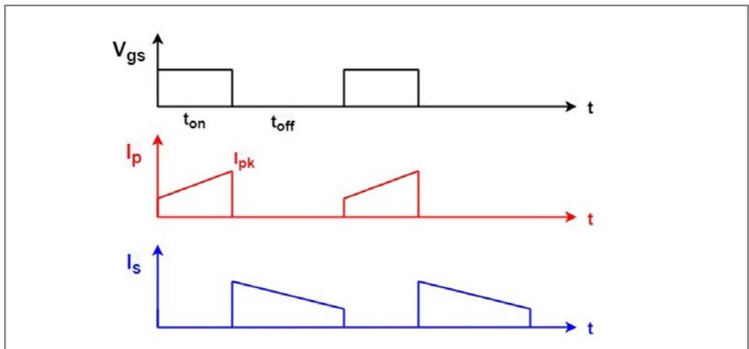
Figure 2 - Flyback main voltage and current waveforms
