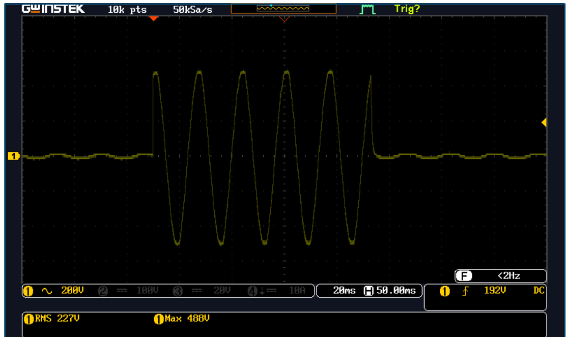
Figure 2. | Five-Cycles of Swell Voltage Bypassing Without Affecting IsoMOV™ Hybrid Protector Operation
