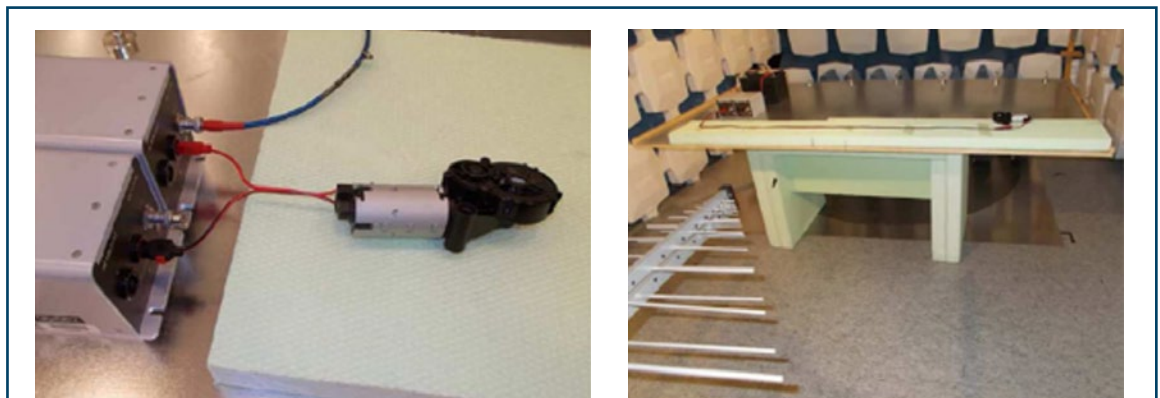
Figure 8. Setup for noise emission test
